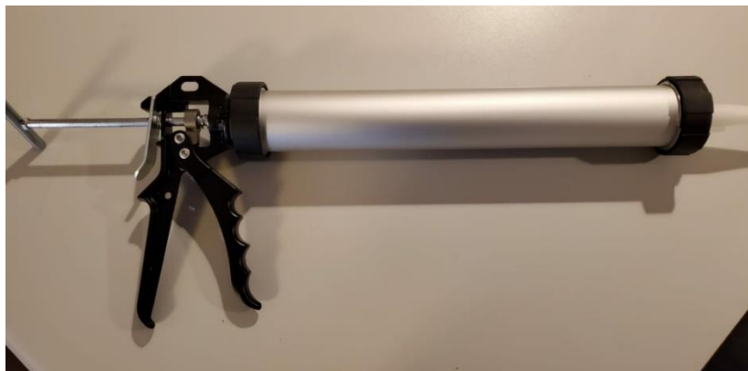
Figure 1: the gun dispenser that will dispense the cocoyam
